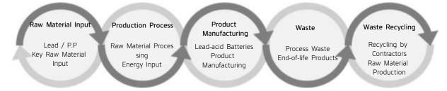
For the main raw and subsidiary materials, including lead and PP (polypropylene), sulfuric acid is used twice during the manufacturing process. The sulfuric acid used in the formation process is fully recycled; this is handled internally. To expand the use of recycled raw materials for key raw and subsidiary materials, we are focusing on establishing a sustainable resource recycling system and are conducting various research and development activities.
